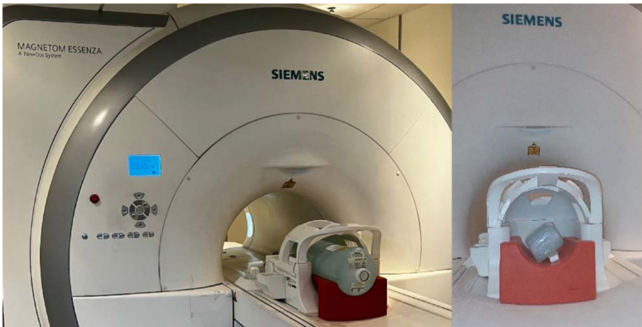
Fig.1: MAGNETOM ESSENZA with Tim + Dot system 1.5 Teslas and two homogenous water phantom inside 16-channel Head/Neck coil. The right image includes the circular phantom that used for SNR measurements, and the left image includes rectangular phantom used for resolution determination.
